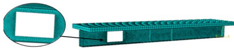
Figure 7 Mesh made for the calibration of the composite beams
