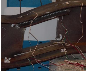
Figure 23 Deformation at the web opening
